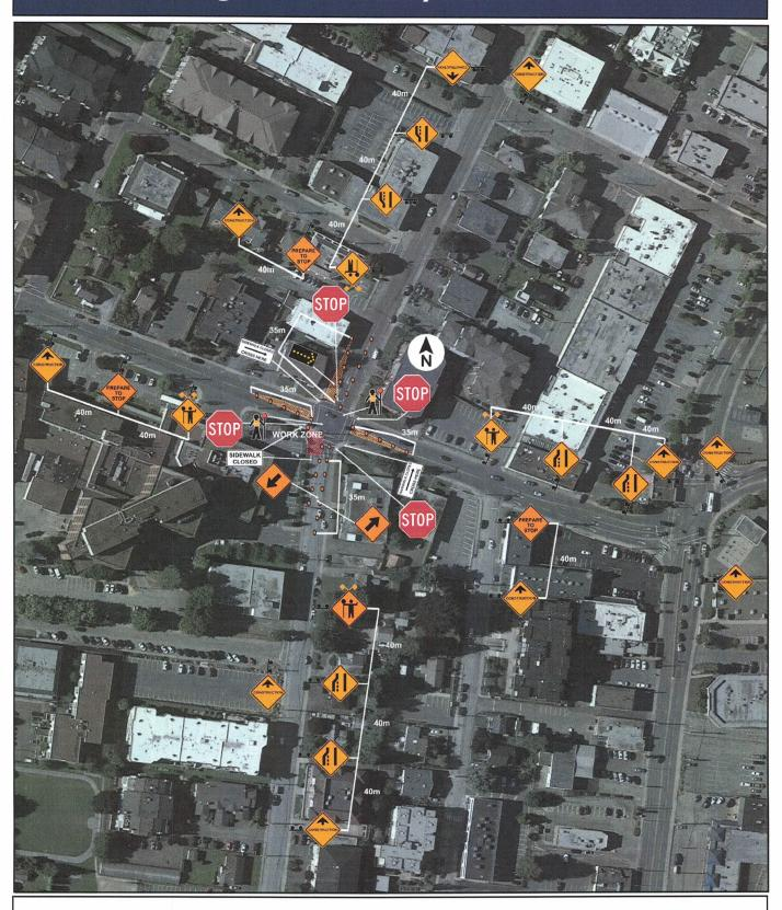
Traffic signals to be turned off for part of construction. 4 Stop signs will be placed at the intersection for four way stop procedure. TCPs to control traffic in the intersection and escort pedestrians safely through work zone.
